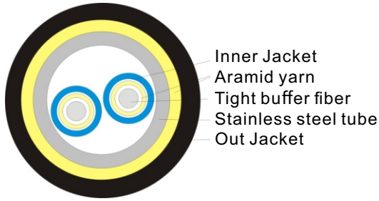
Armored fiber optic cable—Ø7.0mm base stand fiber cable
